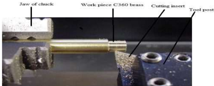
Fig. 4.4:Turning of C360 on CNC lathe
